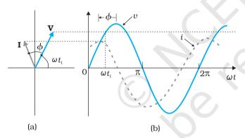
**FIGURE 7.13** (a) Phasor diagram of **V** and **I**. (b) Graphs of v and i versus  $\omega t$  for a series LCR circuit where  $X_C > X_L$ .
