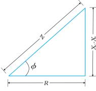
**FIGURE 7.12** Impedance diagram.
