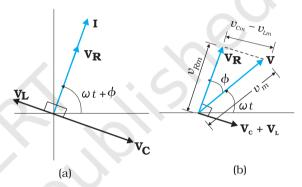
**FIGURE 7.11** (a) Relation between the phasors  $\mathbf{V}_{L}$ ,  $\mathbf{V}_{R}$ ,  $\mathbf{V}_{C}$ , and I, (b) Relation between the phasors  $\mathbf{V}_{L}$ ,  $\mathbf{V}_{R}$ , and  $(\mathbf{V}_{L} + \mathbf{V}_{C})$  for the circuit in Fig. 7.10.
