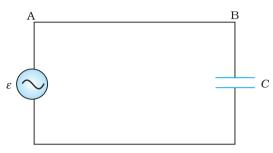
**FIGURE 7.7** An ac source connected to a capacitor.
