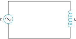
**FIGURE 7.5** An ac source connected to an inductor.
