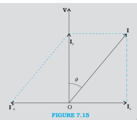
how this can be achieved. Let us resolve  $\mathbf{I}$  into two components.  $\mathbf{I}_p$  along the applied voltage  $\mathbf{V}$  and  $\mathbf{I}_q$  perpendicular to the applied voltage.  $\mathbf{I}_q$  as you have learnt in Section 7.7, is called the wattless component since corresponding to this component of current, there is no power loss.  $\mathbf{I}_p$  is known as the power component because it is in phase with the voltage and corresponds to power loss in the circuit.
